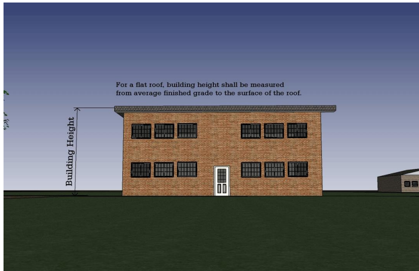
Figure 3.16: Building Height with Flat Roof
