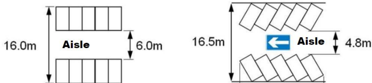
Figure 3.2: Examples of Parking Aisle
